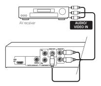
• You can use the SCART AV connector, or the S-video or component video jacks to connect to the AV receiver if you prefer.
